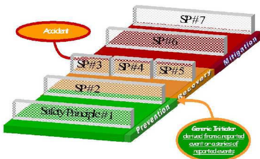
Figure 2: Safety Architecture (i.e. combinations of Safety Principles) associated with a Generic Initiator
